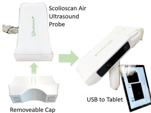
Figure 12. System diagram of the Scolioscan Meter
